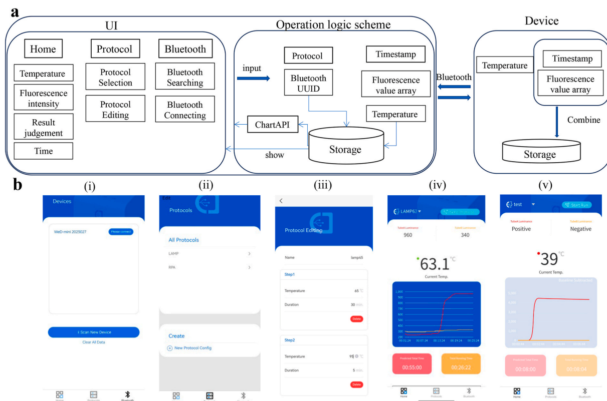
Fig. 2. Overview of the Smartphone App for Device Control and Data Analysis. (a) The architecture of the App includes the user interface (UI), operational logic scheme, and communication with devices. (b) Screenshots of the App interface, featuring: (i) The Bluetooth connection page, (ii) Protocol setting page, (iii) Protocol editing page, (iv) Home page displaying real-time data, and (v) Interface demonstrating automatic result judgment after the reaction.
